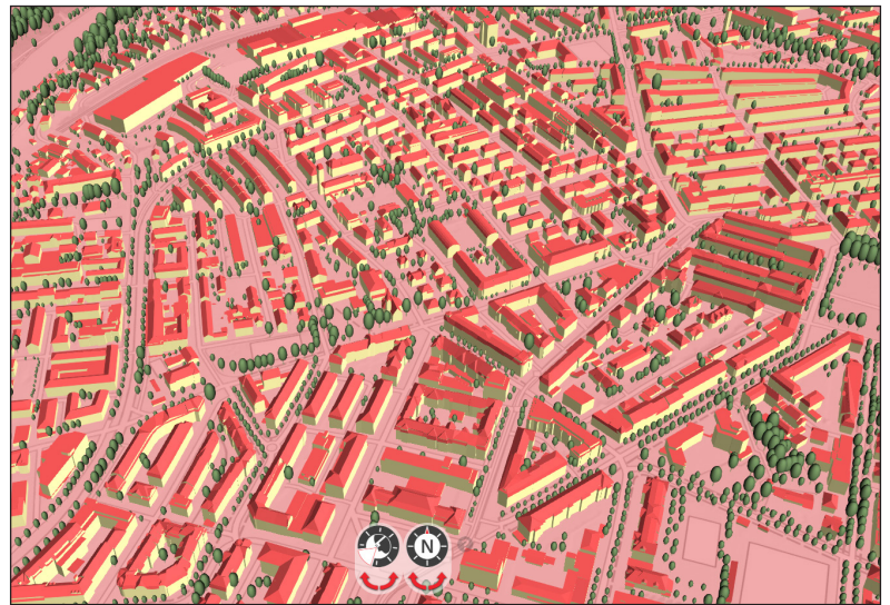
Figure 28 – swissBUILDINGS3D 2.0 model of buildings use photogrammetric capturing method for a high level of precision and detail. Source: Federal Office of Topography (swisstopo) web page.
