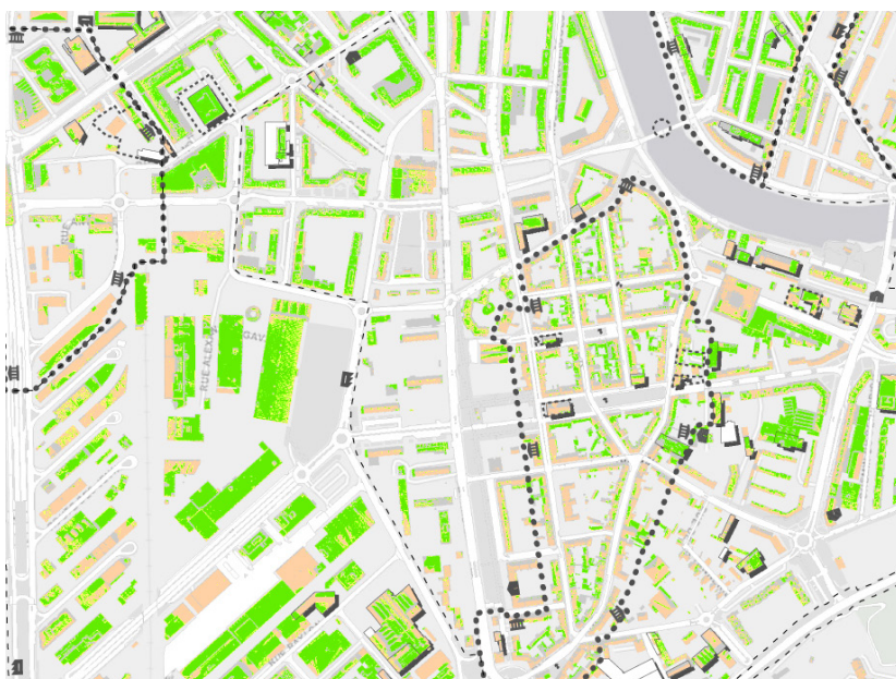
Figure 42: Roof suitability analysis in Geneva, extraction of Carouge district. Roof surfaces are classified by a combination of insulation and visibility thresholds (CHECKMATRIX). Highly sensitive areas are surrounded by thick dashed lines and listed buildings by a contour and a shadow effect.
