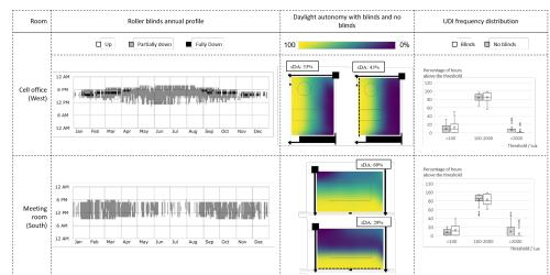
Figure 5. Simulated spatial Daylight Autonomy (sDA) and Useful Daylight Illuminance (UDI) for two spaces and two hypothetic scenarios: 1) no roller blinds in use, and 2) manually operated roller blinds with annual use profile as in figure.
