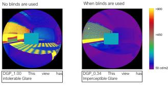
Figure 6. DGP analysis with and without roller blinds for the west facing office. Analysis performed for June  $24^{\rm th}$  at 19:00.
