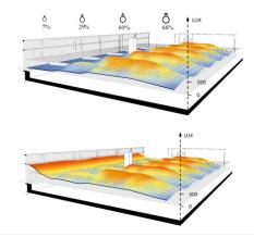
Figure 2. Average and median Daylight Factor(s), and daylight uniformity ratio under overcast conditions for the three monitored spaces: landscape office, west facing and south facing private offices.
