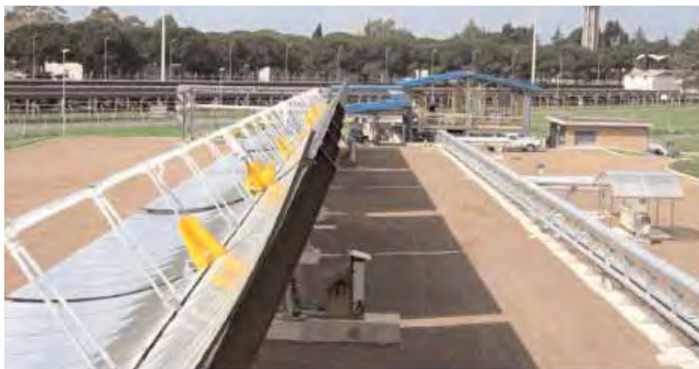
Figure 1. The PCS (Prova Collettori Solari) facility operating in the ENEA Casaccia Research Centre. It consists of two parabolic linear collector 50 m long having an overall collecting area of about 600 m 2 . The heat transfer fluid flowing through the collector is a mixture of molten salt (40% KNO 3 60% NaNO 3 ). The PCS main parameters are: operating temperature 270-550°C, heat transfer fluid flow rate 3.0-7.5 kg/s, molten salt volume 5 m 3 , peak thermal power 500 kW.
