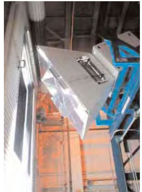
200 kW Solar Simulator at the National Solar Test Facility.
