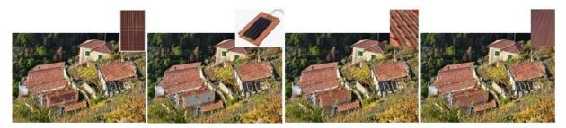
Figure 127: Fossola, simulation of use of different products: coloured PV cells, PV tiles, PV curved tiles, solar copper.
