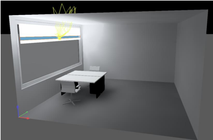
Room illumination by LED Light Guide (LG)
